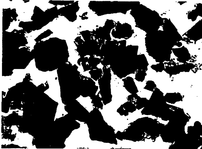
Fig. 24. Sample V.13. Plate-like particles with a few compact types. No fibres present. x 3000
